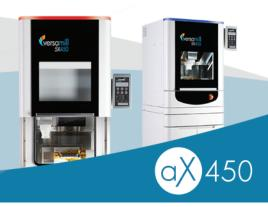
The flagship of our Versamill® compact-machine lineup is our Versamill AX450 precision dental machining center. The AX450 is designed to perform reliably with high precision for the long term. Optomized for custom abutment fabrication from pre-milled blanks, it can process any dental material from zirconia and PMMA to delicate glass ceramics— and even titanium CAD/CAM discs.
